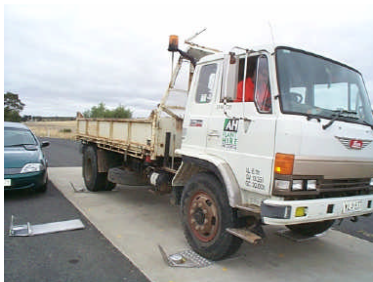
Figure 18: Rigid vehicle being weighed with portable scales
