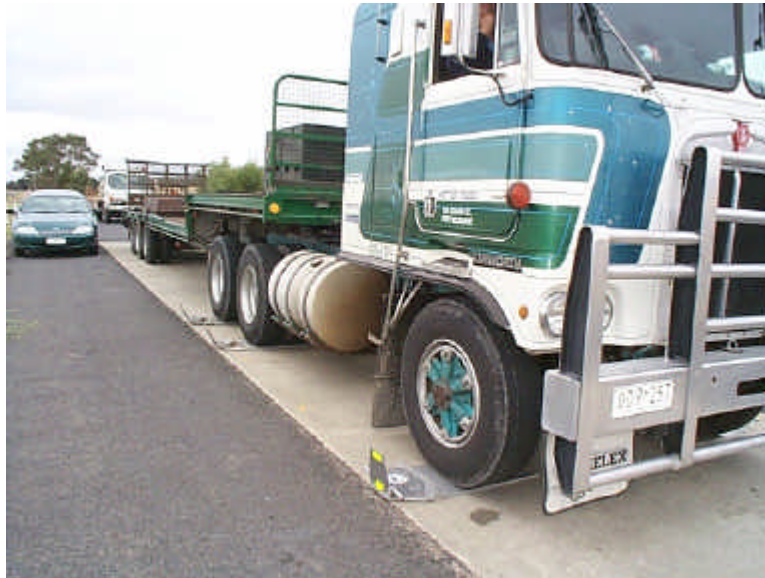
Figure 17: This photo shows 6 scales being used to weigh the steer and tandem drive axles together. Once these axles have been weighed the vehicle is moved and scales are repositioned to weigh the tri-axle group.
