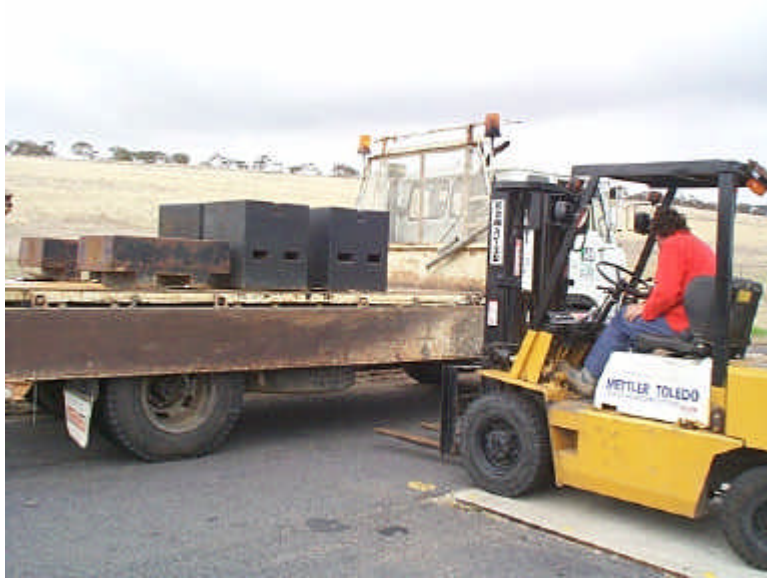
Figure 14: One method is to use a forklift to load steel blocks
